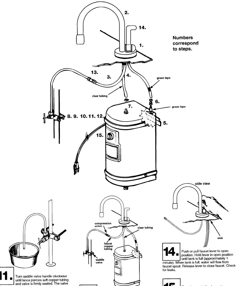
and valve is firmly seated. The valve is now in the closed position. Place a bucket under open end of water supply line. Turn on main water supply valve to pressurize cold water line. Check for leaks. Use a wrench to tighten nut/seal around valve stem.
